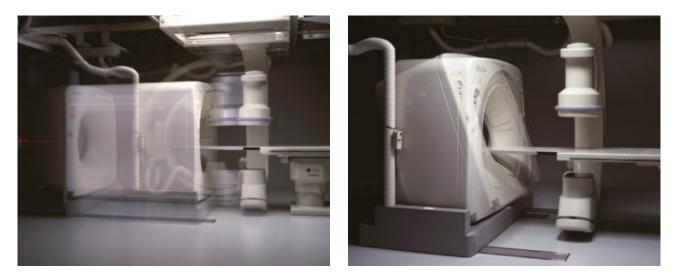
The CT base can move on the floor to realize the helical scan. This unique concept was born by Toshiba/Canon in 1996.
