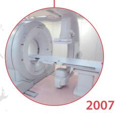
Wider bore permitted easier needle procedure under CT fluoroscopy.
