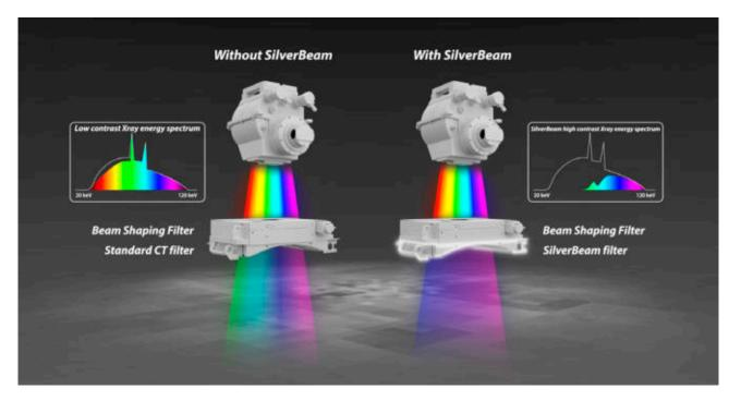
SilverBeam, leverages the photo-attenuating properties of silver to selectively remove photons from a polychromatic x-ray beam leaving an energy spectrum designed for low dose lung screening as shown in the image above.
